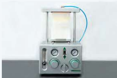
2. Filter with Positive Pressure 24 Processor.
